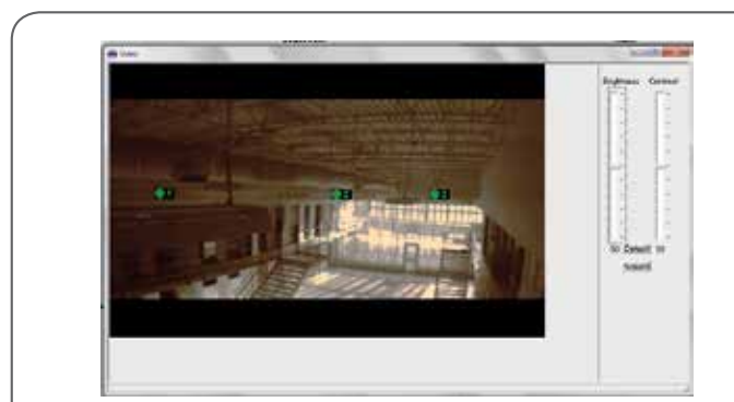
Actual view from the Imager indicating with icons the position of the various Emitters in its field of view
